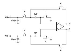
Figure 5. Switched Capacitor Input
