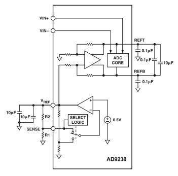
Figure 9. Programmable Reference Configuration
