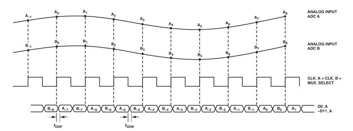
Figure 7. Example of Multiplexed Data Format Using the Channel A Output and the Same Clock Tied to CLK\_A,
