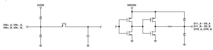
Figure 2. Equivalent Analog Input Circuit
