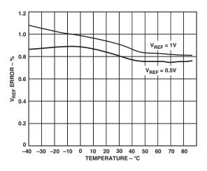
Figure 10. Typical V<sub>REP</sub> Drift
