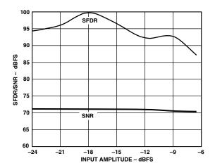
TPC 16. Dual-Tone SNR/SFDR vs. AlN with  $f_{IN}$ 1 = 45 MHz and  $f_{IN}$ 2 = 46 MHz
