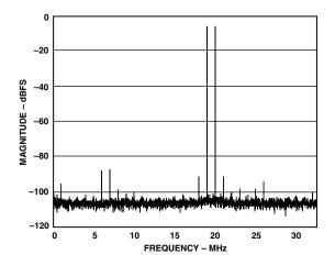
TPC 13. Dual-Tone FFT with  $f_{IN}1 = 45$  MHz and  $f_{IN}2 = 46$  MHz
