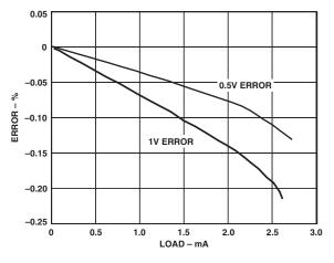
Figure 11. V<sub>RER</sub> Accuracy vs. Load
