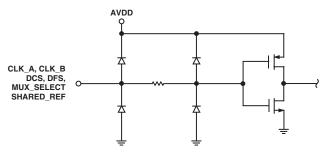
Figure 4. Equivalent Digital Input Circuit
