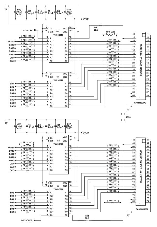
Figure 15. Evaluation Board Schematic (continued)
