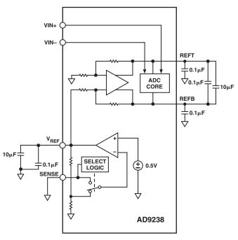
Figure 8. Internal Reference Configuration
