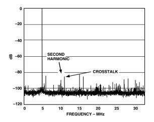
TPC 2. Single-Tone FFT of Channel A Digitizing  $f_{IN} = 70$  MHz while Channel B is Digitizing  $f_{IN} = 76$  MHz
