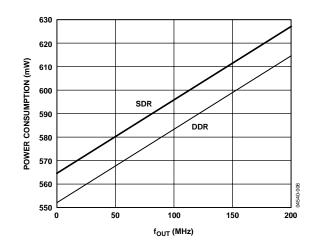
Figure 9. Power Consumption vs. four @ 400 MSPS
