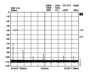
Figure 11. THD @ 400 MSPS and four = 1 MHz (Diplexer High-Pass Output Showing Harmonics Before Calibration; See Performance Effects of Calibration Section)
