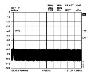
Figure 10. THD @ 400 MSPS and f<sub>OUT</sub> = 1 MHz (Diplexer Low-Pass Output Showing 0 dBm Fundamental; See Performance Effects of Calibration Section)
