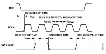
Figure 4. SPI Timing Diagram
