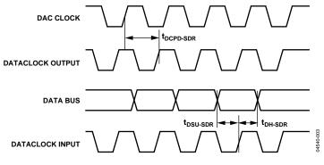
Figure 3. SDR Timing Diagram
