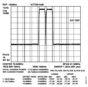
Figure 14. Two-Carrier WCDMA @ 400 MSPS fout = 70 MHz
