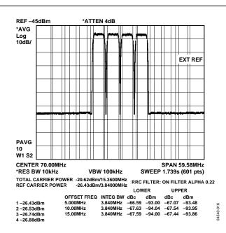
Figure 15. Four-Carrier WCDMA @ 400 MSPS four = 70 MHz
