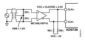
Figure 17. Active DAC Clock Drive Circuit
