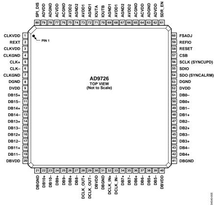
Figure 5. Pin Configuration
