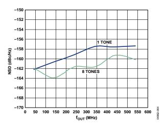
Figure 64. AD9735 NSD vs. f<sub>OUT</sub>, 1.2 GSPS
