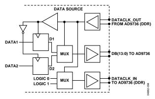
Figure 94. Recommended FPGA/ASIC Configuration for Driving AD973x Digital Inputs, 1× Mode
