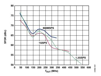
Figure 61. AD9734 SFDR vs. fout over fDAC, 1.2 GSPS
