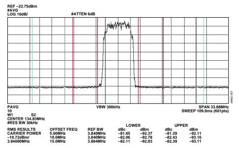
Figure 57. AD9736 WCDMA Carrier at 134.83 MHz,  $f_{DAC} = 491.52$  MSPS
