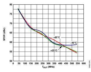
Figure 40. AD9736 SFDR vs. f<sub>OUT</sub> over Temperature
