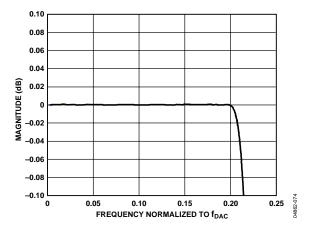
Figure 74. AD973x Interpolation Filter Pass-Band Flatness
