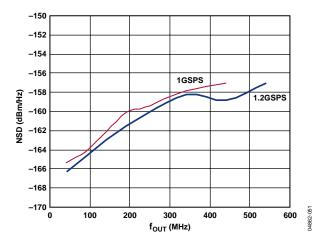
Figure 51. AD9736 1-Tone NSD vs. four over fdac, 25°C
