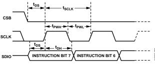
Figure 71. Timing Diagram for SPI Register Write
