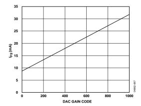
Figure 87. IFS vs. DAC Gain Code
