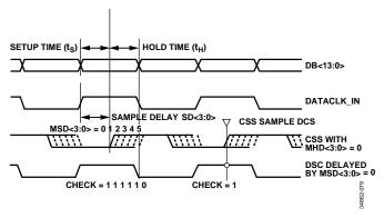
Figure 79. Hold Delay Measurement
