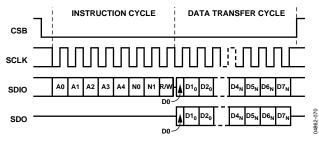
Figure 70. Serial Register Interface Timing, LSB-First Read
