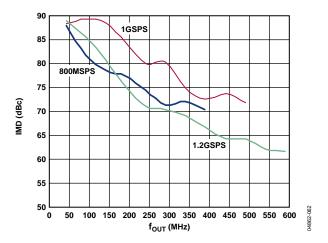
Figure 62. AD9735 IMD vs.  $f_{OUT}$  over  $f_{DAC}$ , 1.2 GSPS
