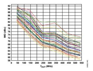
Figure 42. AD9736 IMD vs.  $f_{OUT}$  over 50 parts, 25°C,1.2 GSPS
