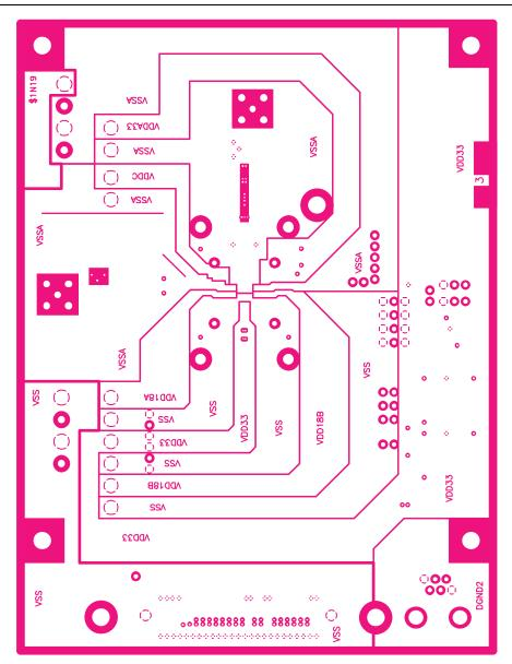
Figure 110. PCB Layout Layer 3, AD973x Evaluation Board, Rev. F
