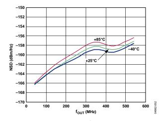
Figure 52. AD9736 1-Tone NSD vs.  $f_{OUT}$  over Temperature, 1.2 GSPS
