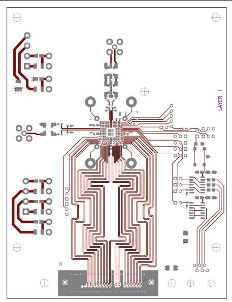
Figure 108. PCB Layout Layer 1, AD973x Evaluation Board, Rev. F
