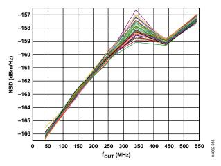
Figure 55. AD9736 1-Tone NSD vs.  $f_{\rm OUT}$  over 50 Parts, 1.2 GSPS, 25°C
