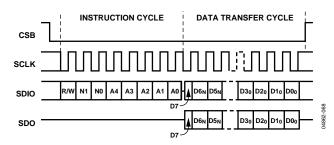
Figure 68. Serial Register Interface Timing, MSB-First Read
