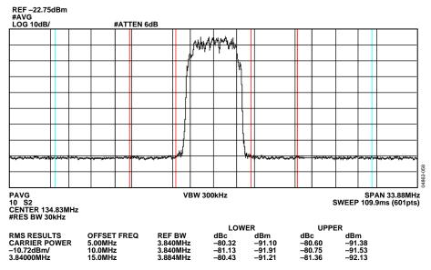
Figure 58. AD9735 WCDMA Carrier at 134.83 MHz,  $f_{DAC} = 491.52$  MSPS
