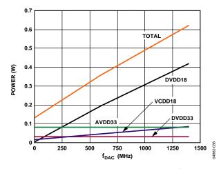
Figure 38. AD9736, 2× Interpolation Mode Power vs. f<sub>DAC</sub> at 25°C
