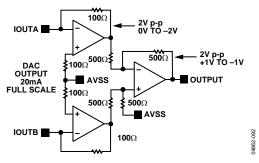
Figure 92. Op Amp I to V Conversion Output Circuit
