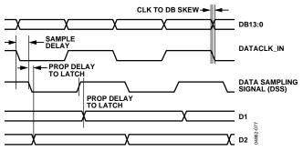
Figure 77. AD973x Internal LVDS Data Sampling Logic Timing
