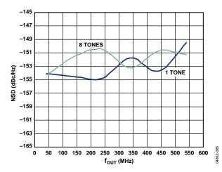
Figure 65. AD9734 NSD vs. fout, 1.2 GSPS
