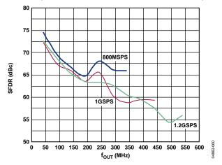
Figure 60. AD9735 SFDR vs. fout over fDAC, 1.2 GSPS
