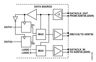
Figure 96. Recommended FPGA/ASIC Configuration for Driving AD973x Digital Inputs, 2× Mode
