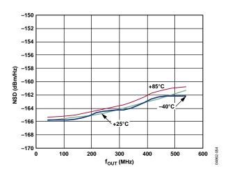
Figure 54. AD9736 8-Tone NSD vs.  $f_{OUT}$  over Temperature, 1.2 GSPS
