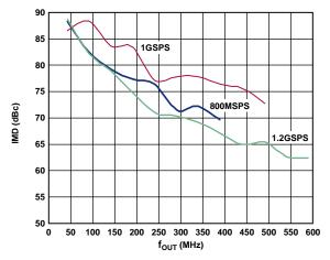
Figure 63. AD9734 IMD vs. fout over fDAC, 1.2 GSPS
