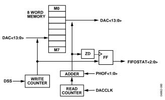
Figure 80. Sync Logic Block Diagram
