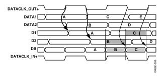
Figure 95. FPGA/ASIC Timing for Driving AD973x Digital Inputs, 1× Mode
