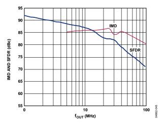
Figure 45. AD9736 Low Frequency IMD and SFDR vs. f<sub>OUT</sub>, 25°C, 1.2 GSPS
