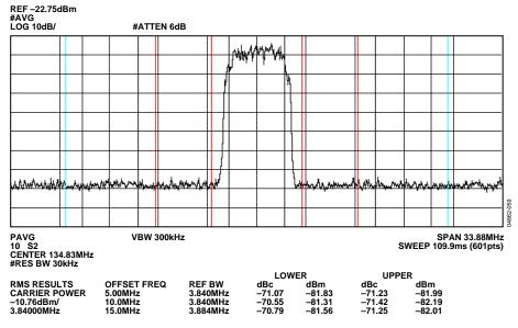
Figure 59. AD9734 WCDMA Carrier at 134.83 MHz,  $f_{DAC} = 491.52$  MSPS
