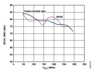
Figure 46. AD9736 IMD and SFDR vs. f<sub>OUT</sub>, 25°C, 1.2 GSPS, 2× Interpolation
