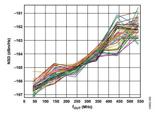
Figure 56. AD9736 1-Tone NSD vs. f<sub>OUT</sub> over 50 Parts, 1.2 GSPS, 25℃
