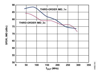
Figure 50. AD9736 IMD vs.  $f_{OUT}$ , 25°C, 1.2 GSPS, 1× and 2× Interpolation
