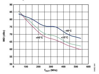
Figure 44. AD9736 IMD vs. fout over Temperature, 1.2 GSPS
