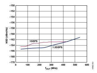
Figure 53. AD9736 8-Tone NSD vs. f<sub>OUT</sub> over f<sub>DAC</sub>, 25°C
