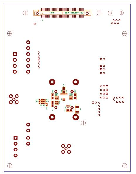
Figure 112. PCB Layout Bottom Placement, AD973x Evaluation Board, Rev. F
