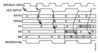
Figure 97. FPGA/ASIC Timing for Driving AD973x Digital Inputs, 2× Mode
