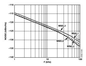
Figure 85. 1/f Noise with Respect to MSEL Bits
