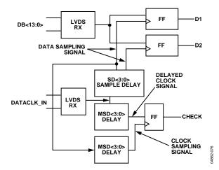
Figure 76. AD973x Internal LVDS Data Sampling Logic
