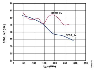
Figure 49. AD9736 SFDR vs. f<sub>OUT</sub>, 25°C, 1.2 GSPS, 1× and 2× Interpolation
