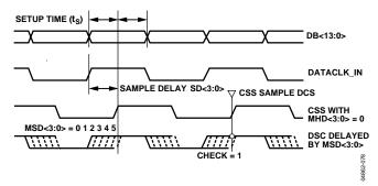
Figure 78. Setup Delay Measurement
