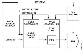
Figure 75. AD973x Data Controllers
