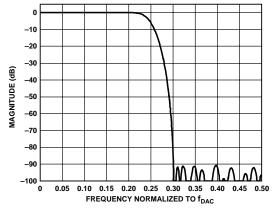
Figure 73. AD973x Interpolation Filter Response
