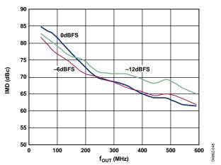
Figure 48. AD9736 IMD vs. f<sub>OUT</sub> over A<sub>OUT</sub>, 25°C, 1.2 GSPS
