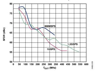
Figure 39. AD9736 SFDR vs. four over fDAC at 25°C
