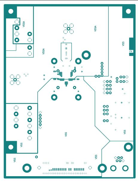
Figure 109. PCB Layout Layer 2, AD973x Evaluation Board, Rev. F
