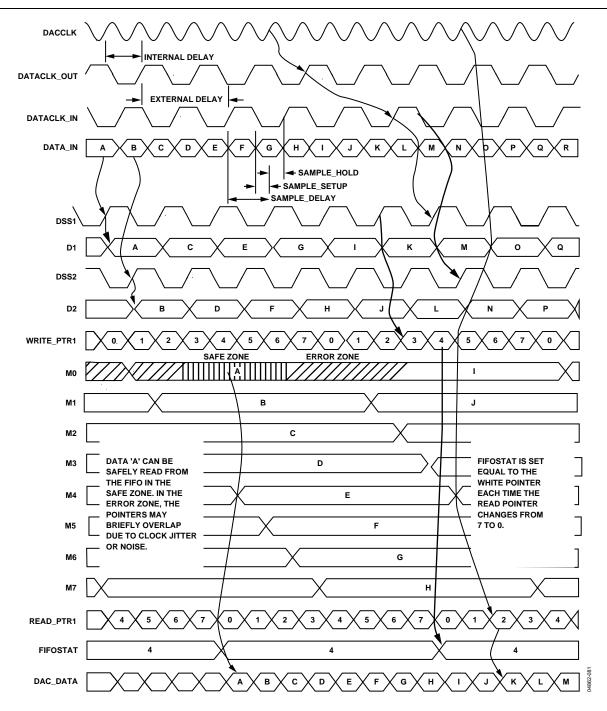
Figure 81. SYNC Logic Timing Diagram
