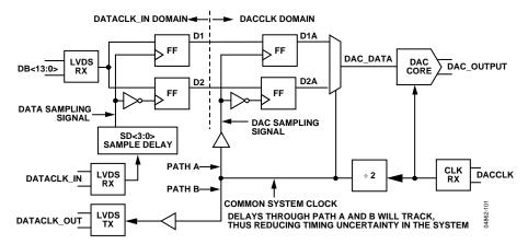
Figure 101. Simplified Internal Clock Routing
