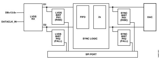
Figure 82. Block Diagram Showing LVDS and Sync Phase 1 and Phase 2
