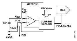
Figure 86. Voltage Reference Circuit
