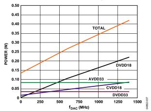
Figure 37. AD9736 1× Mode Power vs.  $f_{DAC}$  at 25°C
