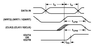
Figure 1. Timing Diagram for Dual and Interleaved Modes
