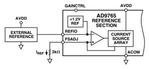
Figure 22. External Reference Configuration
