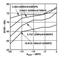
Figure 11. Dual-Tone SFDR vs.  $A_{OUT}$  @  $f_{OUT} = f_{CLOCK}/7$
