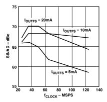
Figure 12. SINAD vs.  $f_{CLOCK}$  and  $I_{OUTFS}$  @  $f_{OUT} = 5$  MHz and 0 dBFS
