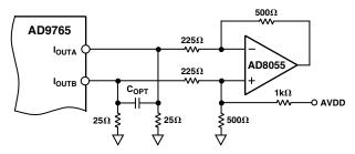
Figure 35. Single Supply DC Differential Coupled Circuit
