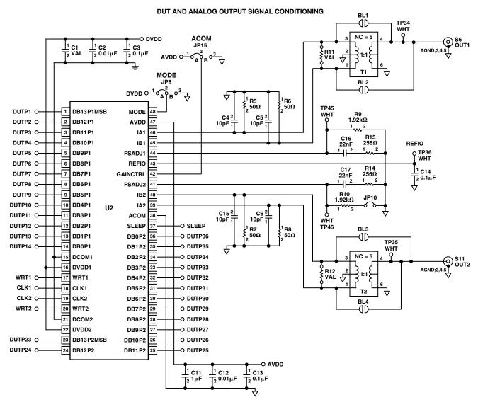
Figure 47. AD9765 and Output Signal Conditioning
