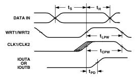
Figure 23. Dual Mode Timing
