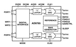
and provide a nominal full-scale current of 20 mA. The full-scale currents between each DAC are matched to within 0.1%.
