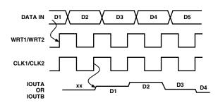
Figure 24. Dual Mode Timing
