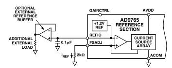
Figure 21. Internal Reference Configuration
