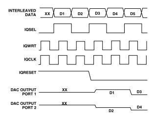
Figure 27. Interleaved Mode Timing
