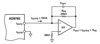
Figure 37. Unipolar Buffered Voltage Output
