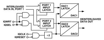
Figure 25. Latch Structure Interleaved Mode
