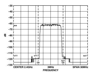
Figure 43. CDMA Signal, 8 M Chips Sampled at 65 MSPS, Recreated at 2.4 GHz, Adjacent Channel Power > 60 dBm
