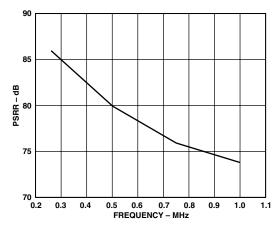
Figure 38. Power Supply Rejection Ratio of AD9765
