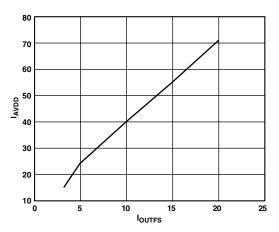
Figure 30. I<sub>AVDD</sub> vs. I<sub>OUTFS</sub>
