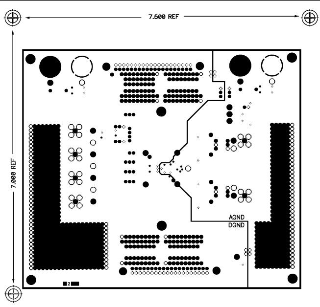
Figure 51. Layer 2, Ground Plane
