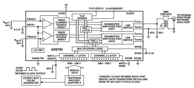
Figure 2. Basic AC Characterization Test Setup for AD9765, Testing Port 1 in Dual Port Mode, Using Independent GAINCTRL Resistors on FSADJ1 and FSADJ2
