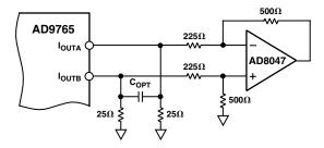
Figure 34. DC Differential Coupling Using an Op Amp
