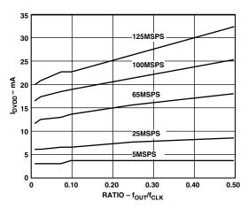
Figure 31.  $I_{DVDD}$  vs. Ratio @ DVDD = 5 V
