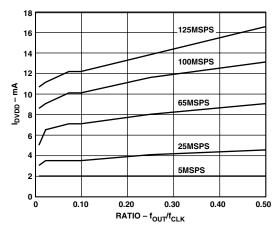
Figure 32. I<sub>DVDD</sub> vs. Ratio @ DVDD = 3 V
