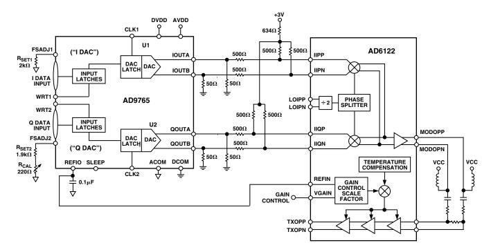
Figure 44. CDMA Transmit Application Using AD9765 and AD6122
