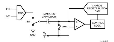
FIGURE 2. ADC082S021 in Hold Mode
