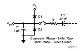
FIGURE 5. Equivalent Input Circuit
