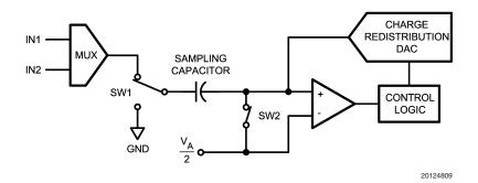
FIGURE 1. ADC082S021 in Track Mode
