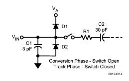
FIGURE 5. Equivalent Input Circuit
