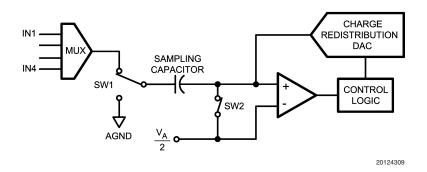
FIGURE 1. ADC124S021 in Track Mode
