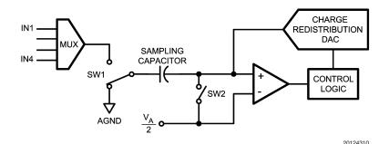
FIGURE 2. ADC124S021 in Hold Mode
