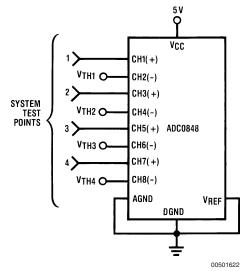
DO = all 1s if  $V_{IN}(+)>V_{IN}(-)$ DO = all 0s if  $V_{IN}(+)< V_{IN}(-)$
