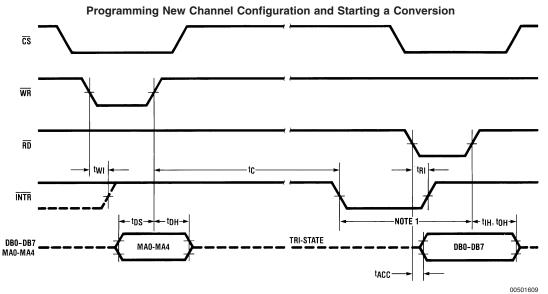
Note 13: Read strobe must occur at least 600 ns after the assertion of interrupt to guarantee reset of  $\overline{\text{INTR}}$  .
