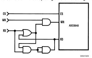
$\overline{\text{CS}}~\bullet\overline{\text{WR}}$  will update the channel configuration and start a conversion.
