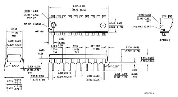
Molded Dual-In-Line Package (N) NS Package Number N20A
