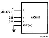
FIGURE 1. Analog Input Multiplexer Options
