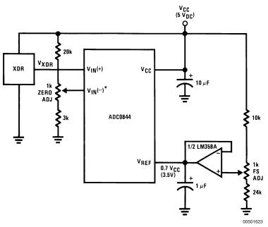
\*  $V_{IN}(-)$ =0.15  $V_{CC}$ 15% of  $V_{CC} \le V_{XDR} \le 85\%$  of  $V_{CC}$
