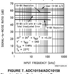
Signal-to-Noise Ratio vs Input Frequency
