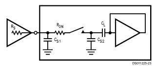
FIGURE 6. Analog Input Model
