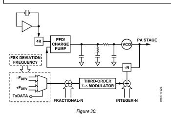
The deviation from the center frequency is set using bits D1 to D9 in the modulation register. The frequency deviation may be set in steps of
