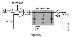
$$F_{OUT} = \frac{F_{CRYSTAL} \times N}{R} = F_{PFD} \times N \tag{1}$$
