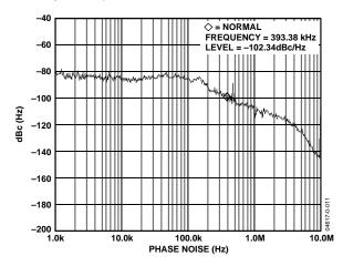
Figure 11. Phase Noise Response— $I_{CP} = 2.0 \text{ mA}$ ,  $I_{VCO} = 2.0 \text{ mA}$ ,  $RF_{OUT} = 433.92 \text{ MHz}$ , PFD = 4 MHz, PA Bias = 5.5 mA
