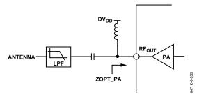
Figure 38. ADF7012 with Harmonic Filter
