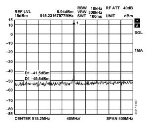
Figure 23. Spurious Components—Meets FCC Specs
