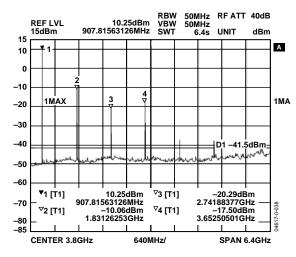
Figure 24. Harmonic Response,  $RF_{OUT}$  Matched to 50  $\Omega$ , No Filter
