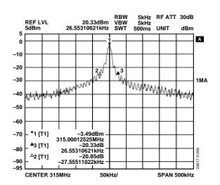
Figure 9. OOK Modulation, Power = 0 dBm, Data Rate = 10 kbps
