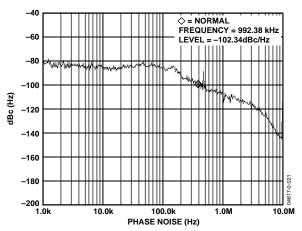
Figure 21. Phase Noise Response– $l_{CP}$  = 1.44 mA,  $l_{VCO}$  = 3.0 mA,  $RF_{OUT}$  = 915.2 MHz, PFD =10 MHz, Power = 10 dBm, PA Bias = 5.5 mA
