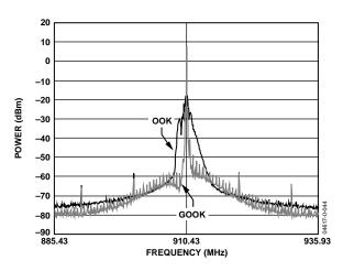
Figure 34. GOOK vs. OOK Frequency Spectra (Wideband Measurement)
