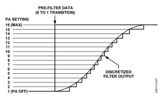
Figure 32. Varying PA Output for GOOK (Index Counter = 16).
