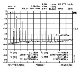
Figure 7. Harmonic Response, RF<sub>OUT</sub> Matched to 50 Ω, No Filter
