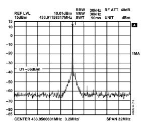
Figure 13. Spurious Components—Meets ETSI Specs
