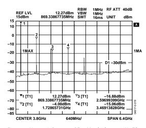
Figure 19. Harmonic Response,  $RF_{OUT}$  Matched to 50  $\Omega$ , No Filter
