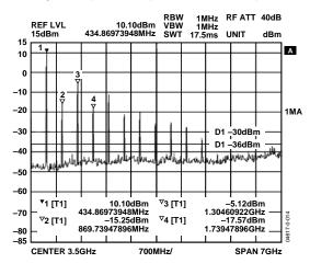
Figure 14. Harmonic Response,  $RF_{OUT}$  Matched to 50  $\Omega$ , No Filter
