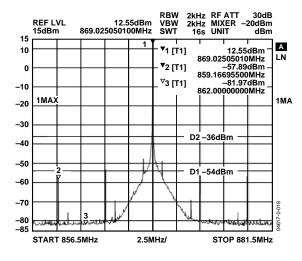
Figure 18. Spurious Components—Meets ETSI Specs
