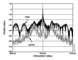
Figure 33. GOOK vs. OOK Frequency Spectra (Narrow-Band Measurement)
