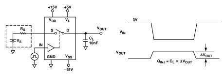
Test Circuit 6. Charge Injection
