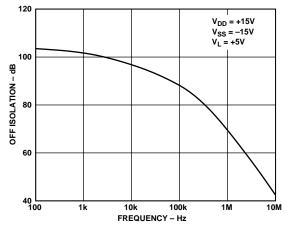
Figure 7. Off Isolation vs. Frequency
