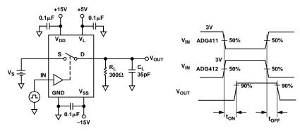
Test Circuit 4. Switching Times
