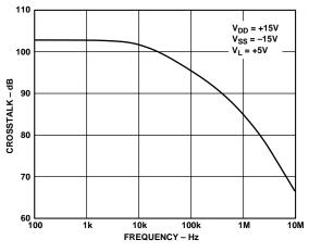
Figure 8. Crosstalk vs. Frequency
