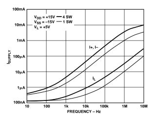
Figure 5. Supply Current vs. Input Switching Frequency
