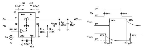
Test Circuit 5. Break-Before-Make Time Delay
