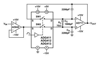
Figure 9. Fast, Accurate Sample-and-Hold
