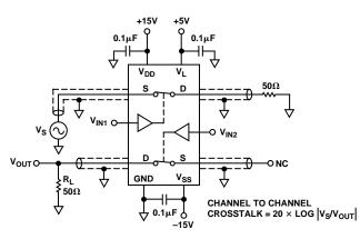
Test Circuit 8. Channel-to-Channel Crosstalk
