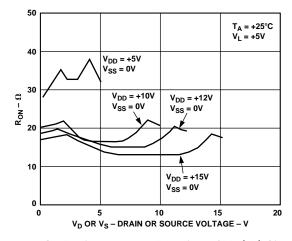
Figure 4. On Resistance as a Function of  $V_{\text{D}}$  (V\_{\text{S}}) Single Supply
