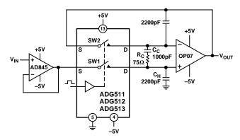
Figure 9. Accurate Sample-and-Hold
