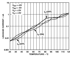
Figure 5. Leakage Currents as a Function of Temperature
