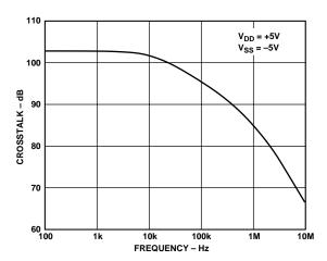
Figure 8. Crosstalk vs. Frequency
