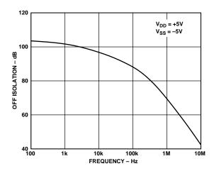
Figure 6. Off Isolation vs. Frequency
