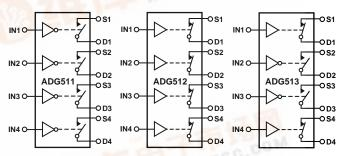
SWITCHES SHOWN FOR A LOGIC "1" INPUT
