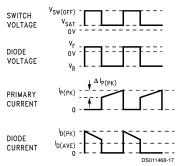
FIGURE 17. Flyback Regulator Waveforms
