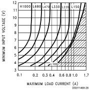
FIGURE 8. LM2577-15 Inductor Selection Guide
