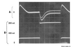
A: Output Voltage Change, 100 mV/div. (AC-coupled) B: Load current, 0.2 A/div
