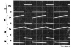
A: Switch pin voltage, 10 V/div
