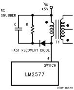
FIGURE 21. Snubber Circuit
