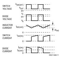
FIGURE 5. Step-Up Regulator Waveforms
