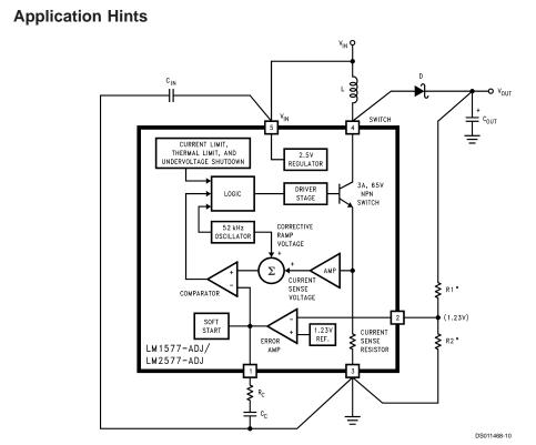
Note: Pin numbers shown are for TO-220 (T) package \*Resistors are internal to LM1577/LM2577 for 12V and 15V versions.
