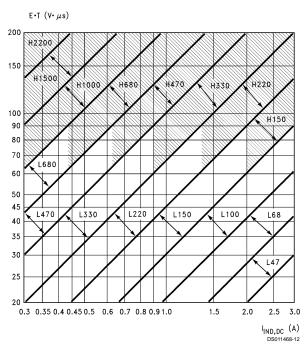
**Note:** These charts assume that the inductor ripple current inductor is approximately 20% to 30% of the average inductor current (when the regulator is under full load). Greater ripple current causes higher peak switch currents and greater output ripple voltage; lower ripple current is achieved with larger-value inductors. The factor of 20 to 30% is chosen as a convenient balance between the two extremes.
