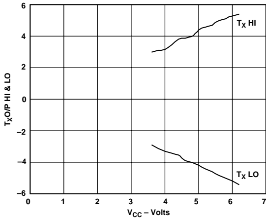
Figure 4. Tx Output Voltage vs. Supply
