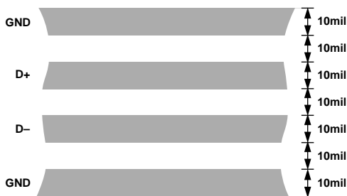
Figure 14. Arrangement of Signal Tracks
