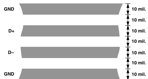
Figure 17. Arrangement of Signal Tracks
