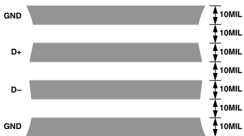
Figure 15. Arrangement of Signal Tracks
