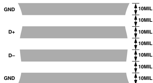
Figure 12. Arrangement of Signal Tracks
