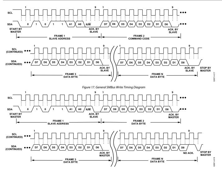
Figure 18. General SMBus Read Timing Diagram
