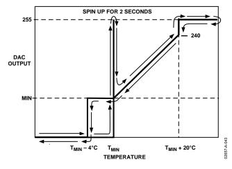
Figure 43. Automatic DAC Fan Control Transfer Function
