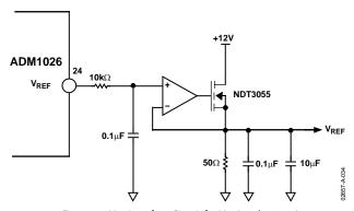
Figure 33.  $V_{REF}$  Interface Circuit for  $V_{REF}$  Loads > 2 mA
