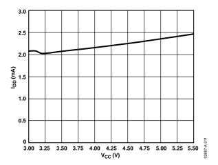
Figure 11. Supply Current vs. Supply Voltage
