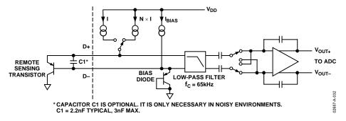
Figure 34. Signal Conditioning for Remote Diode Temperature Sensors
