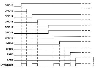
Figure 61. NAND Tree Test with Two Inputs Shorted
