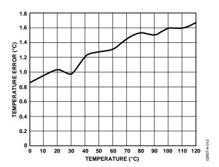
Figure 12. Local Sensor Temperature Error
