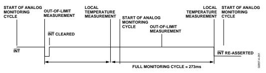
Figure 50. Delay After Clearing INT Before Reassertion
