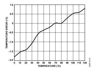
Figure 13. Remote Sensor Temperature Error
