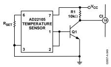
Figure 49. Using the CI Input with a Temperature Sensor
