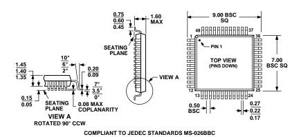
Figure 63. 48-Lead Thin Plastic Quad Flat Package [LQFP] 7 mm x 7 mm x 1.4 mm Thick (ST-48) Dimensions shown in millimeters
