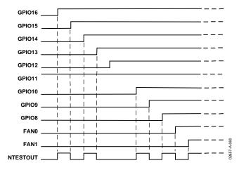
Figure 60. NAND Tree Test with One Input Stuck High
