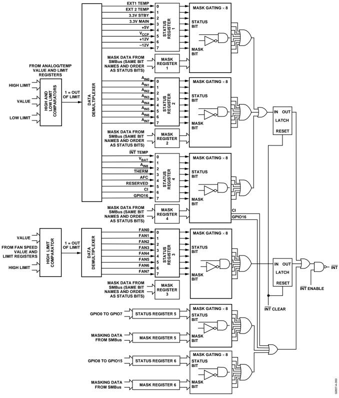
Figure 53. Interrupt Structure
