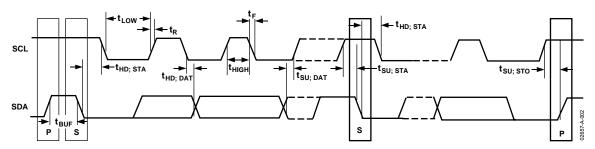
Figure 2. Serial Bus Timing Diagram
