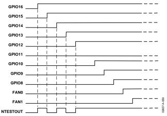
Figure 59. NAND Tree Test with GPIO11 Stuck Low
