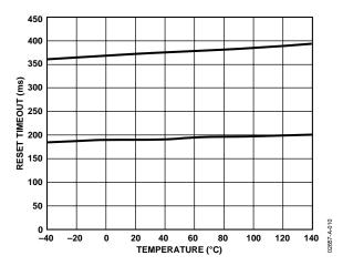
Figure 10. Power-up Reset Timeout vs. Temperature
