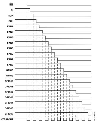
Figure 58. NAND Tree Test Taking Inputs Low in Turn
