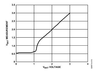
Figure 15.  $V_{BAT}$  Measurement vs. Voltage
