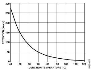
Figure 16. Typical EEPROM Memory Retention
