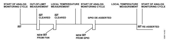
Figure 51. Other Interrupt Sources Can Reassert INT Immediately
