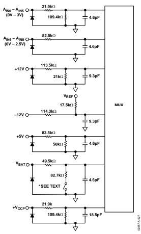
Figure 27. Voltage Measurement Inputs
