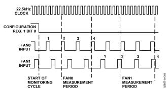
Figure 48. Fan Speed Measurement
