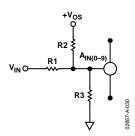
Figure 30. Scaling and Offsetting A<sub>INO</sub> – A<sub>IN9</sub> for Bipolar Inputs
