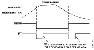
Figure 54. Assertion of INT Due to THERM Event
