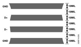
Figure 35. Arrangement of Signal Tracks
