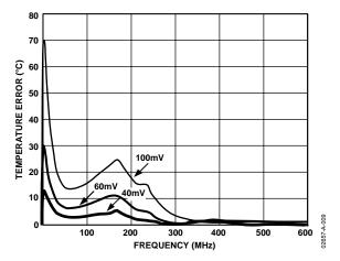
Figure 9. Temperature Error vs. Differential-Mode Noise Frequency
