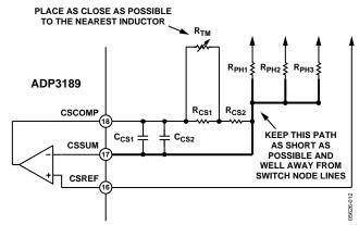
Figure 12. Temperature Compensation Circuit Values
