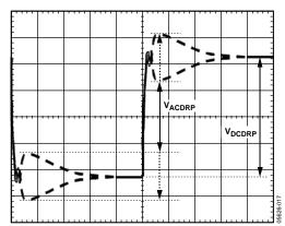
Figure 17. AC Loadline Waveform
