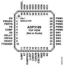
Figure 5. Pin Configuration
