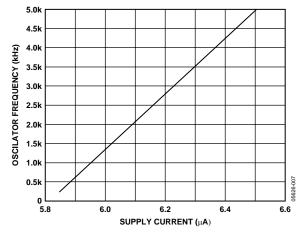
Figure 7. Oscillator Frequency vs . Supply Current
