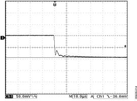
Figure 14. Typical Transient Response for Design Example Load Step
