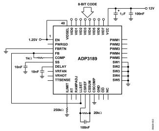
Figure 2. Closed-Loop Output Voltage Accuracy
