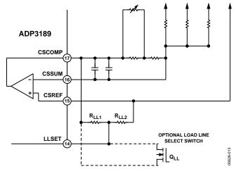
Figure 13. Load Line Setting Resistors
