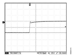
Figure 15. Typical Transient Response for Design Example Load Release
