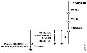
Figure 16. VR Thermal Monitor Circuit
