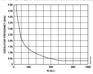
Figure 6. Master Clock Frequency vs. RT
