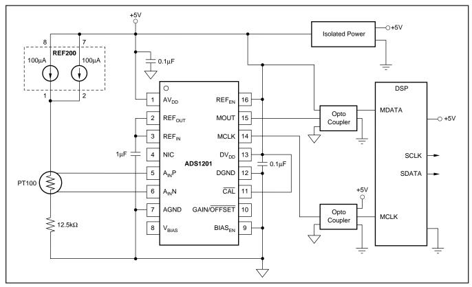
FIGURE 12. PT100 Interface with Current Excitation.
