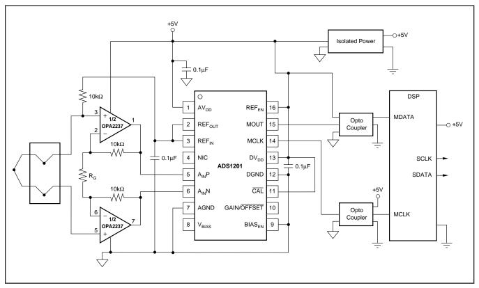
FIGURE 14. Single-Supply, High Accuracy Thermocouple Interface.
