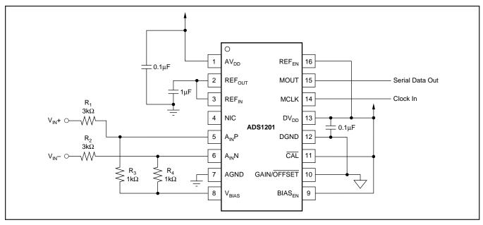
FIGURE 6.  $\pm 10V$  Bipolar Input Configuration Using V<sub>BIAS</sub>.
