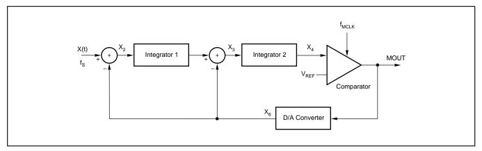
FIGURE 4. Block Diagram of a Second-Order Modulator.
