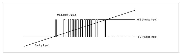
FIGURE 8. Analog Input versus Modulator Output of the ADS1201.
