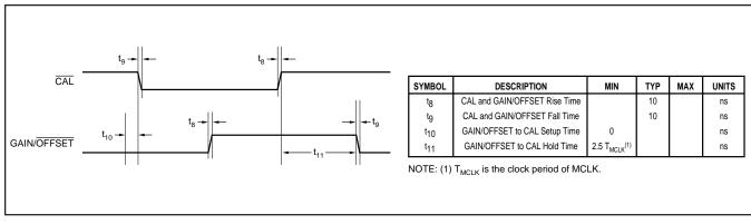
FIGURE 9. Timing Diagram for the Calibration Feature of the ADS1201.
