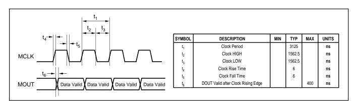
FIGURE 7. Timing Diagram for the Digital Interface of the ADS1201.
