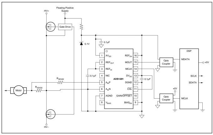
FIGURE 15. Motor Controller Sensing Circuit.
