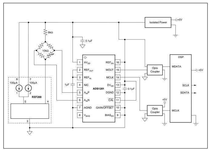
FIGURE 11. Bridge Transducer Interface with Current Excitation.
