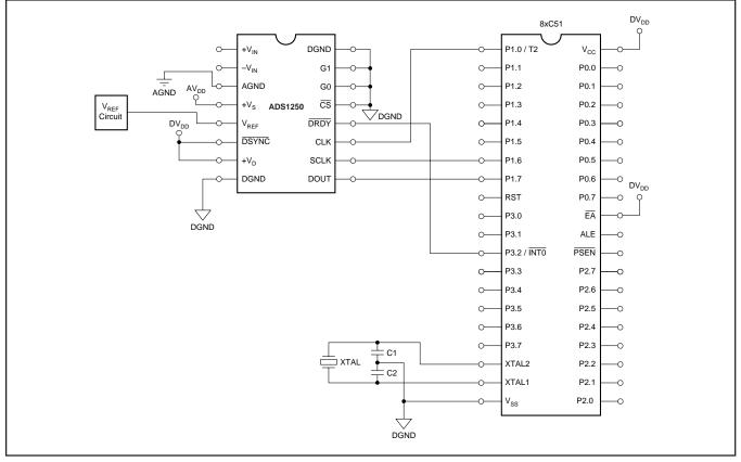
FIGURE 21. Three-Wire Interface to an 8xC51 (CS tied LOW).
