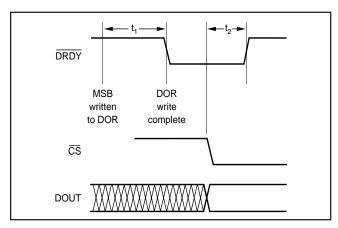
FIGURE 14.  $\overline{DRDY}$  Pulse (using  $\overline{CS}$ ).
