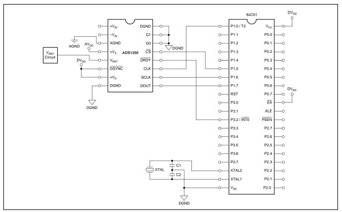
FIGURE 17 Four-Wire Interface to an 8xC51
