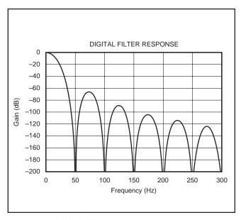
FIGURE 4. Digital Filter Response (50Hz).
