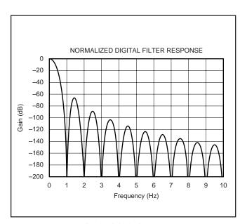
FIGURE 3. Normalized Digital Filter Response.
