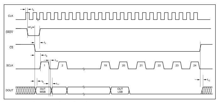
FIGURE 16. Method 1: Four-Wire Interface Using Noncontinuous SCLK.
