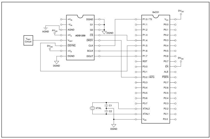
FIGURE 22. Five-Wire Interface to an 8xC51.
