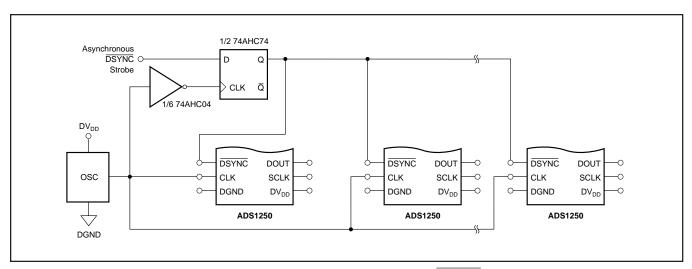
FIGURE 12. Exactly Synchronizing Multiple ADS1250s to an Asynchronous DSYNC Signal.
