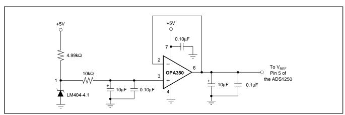
FIGURE 2. Recommended External Voltage Reference Circuit for Best Low Noise Operation with the ADS1250
