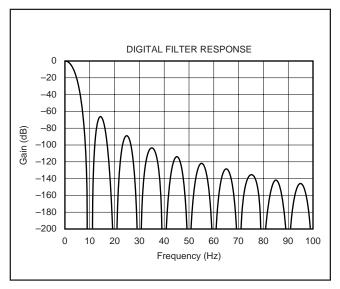
FIGURE 6. Digital Filter Response (10Hz Multiples).
