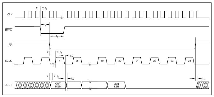
FIGURE 18. Method 2: Four-Wire Interface Using a Free-Running SCLK.
