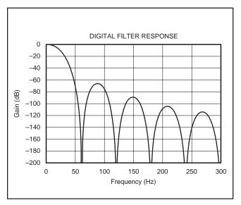
FIGURE 5. Digital Filter Response (60Hz).
