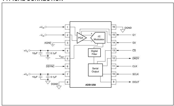
FIGURE 25. Connection Diagram.
