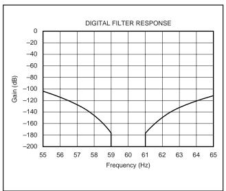
FIGURE 9. Expanded Digital Filter Response (60Hz with a
