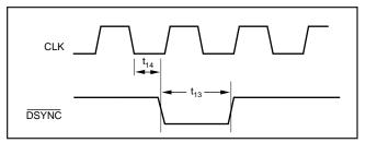
FIGURE 11. DSYNC to CLK Timing for Synchronizing Multiple ADS1250s.
