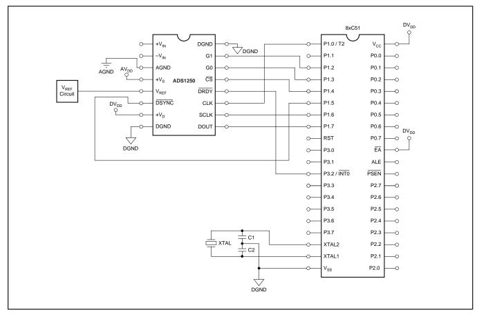
FIGURE 23. Full Interface to an 8xC51.
