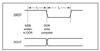
FIGURE 13.  $\overline{DRDY}$  Pulse ( $\overline{CS}$  tied LOW).
