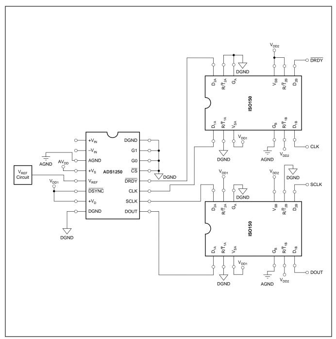
FIGURE 24. Isolated Four-Wire Interface.
