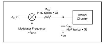
FIGURE 1. Analog Input Structure.
