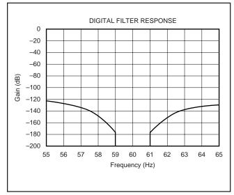
FIGURE 10. Expanded Digital Filter Response (60Hz with
