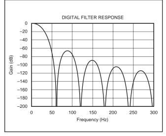
FIGURE 5. Digital Filter Response (60Hz).
