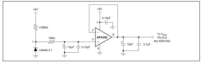
FIGURE 2. Recommended External Voltage Reference Circuit for Best Low Noise Operation with the ADS1252.
