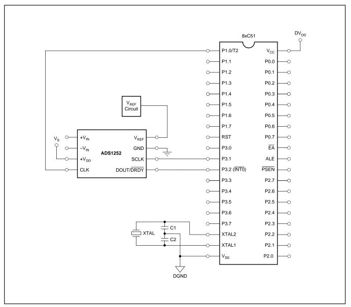
FIGURE 15. Two-Wire Interface to an 8xC51.
