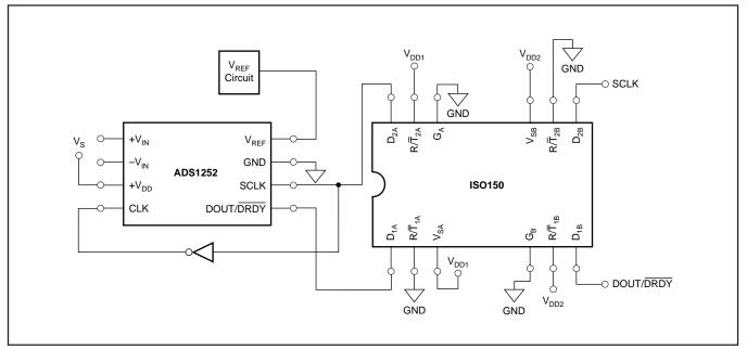
FIGURE 16. Isolated Three-Wire Interface.
