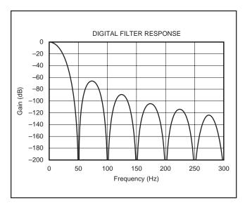
FIGURE 4. Digital Filter Response (50Hz).
