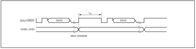
FIGURE 13. Multiplexer Operation.
