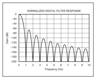
FIGURE 4. Normalized Digital Filter Response.
