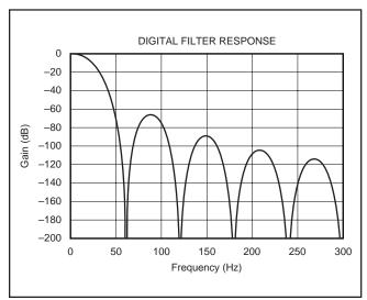
FIGURE 6. Digital Filter Response (60Hz).
