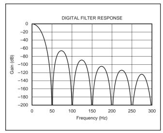
FIGURE 5. Digital Filter Response (50Hz).
