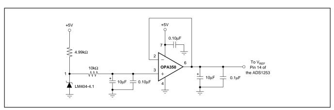
FIGURE 3. Recommended External Voltage Reference Circuit for Best Low-Noise Operation with the ADS1253.
