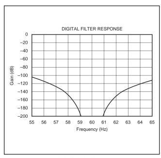
FIGURE 10. Expanded Digital Filter Response (60Hz with a 60Hz Data Output Rate).
