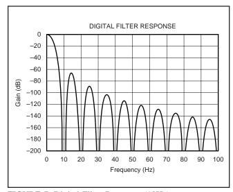
FIGURE 7. Digital Filter Response (10Hz).
