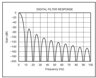
FIGURE 7. Digital Filter Response (10Hz).
