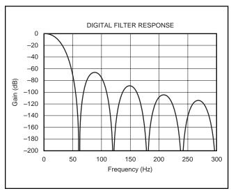
FIGURE 6. Digital Filter Response (60Hz).
