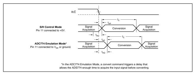
FIGURE 9. Signal Acquisition and Conversion Timing.
