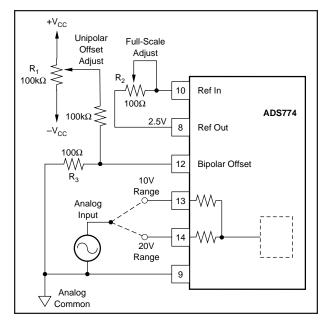
FIGURE 10. Unipolar Configuration.
