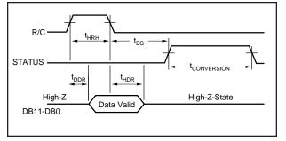
FIGURE 3. R/C Pulse Low—Outputs Enabled After Conversion.
