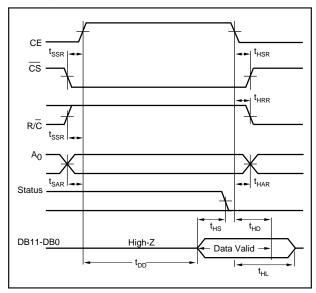
FIGURE 6. Read Cycle Timing.
