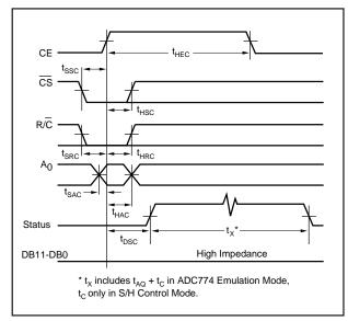
FIGURE 5. Conversion Cycle Timing.
