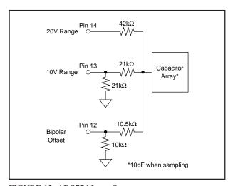
FIGURE 12. ADS774 Input Structure.
