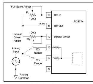
FIGURE 11. Bipolar Configuration.
