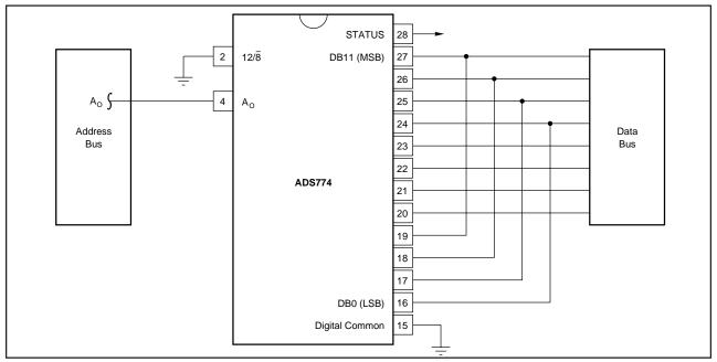
FIGURE 8. Connection to an 8-Bit Bus.
