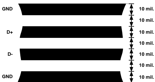
Figure 12. Arrangement of Signal Tracks
