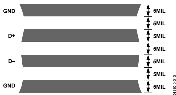
Figure 22. Typical Arrangement of Signal Tracks
