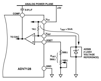
\*ADDITIONAL CIRCUITRY, INCLUDING DECOUPLING COMPONENTS, EXCLUDED FOR CLARITY
