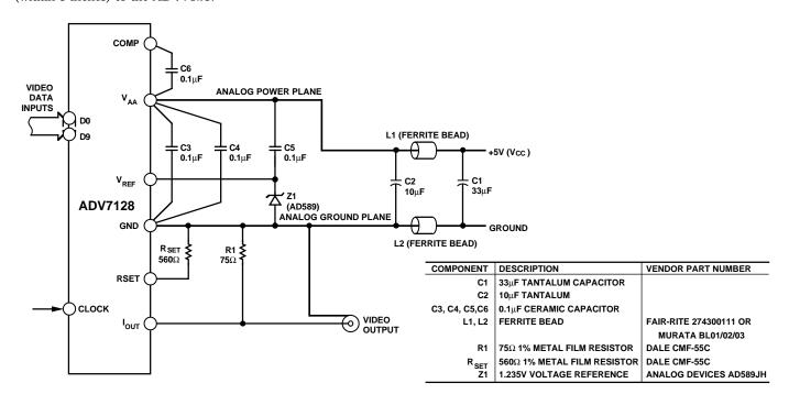
Figure 7. ADV7128 Typical Connection Diagram and Component List
