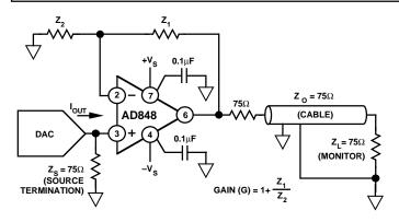
Figure 6. AD848 As an Output Buffer
