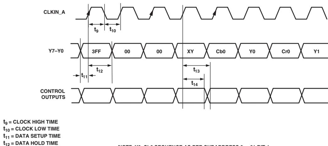
Figure 7. PS Only 4:2:2 1 × 8-Bit Interleaved at 54 MHz EAV/SAV Input Mode [Input Mode 111]
