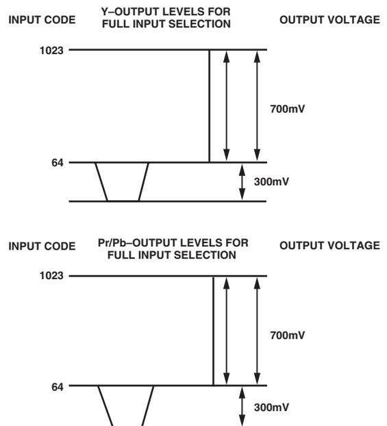
Figure 94. Output Levels for Full Input Selection
