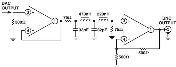
Figure 57. Example of Output Filter for HDTV, 2× Oversampling
