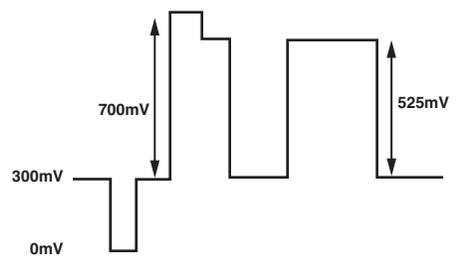
Figure 98. SD RGB Output Levels—RGB Sync Enabled
