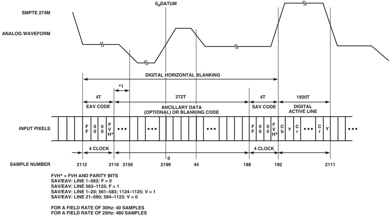
Figure 111. EAV/SAV Input Data Timing Diagram—SMPTE 274M
