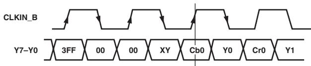
CLOCK EDGE ADDRESS 0x00 BIT 1 SHOULD BE SET TO 0 IN THIS CASE.
