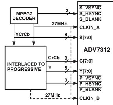
Figure 23. Simultaneous PS and SD Input
