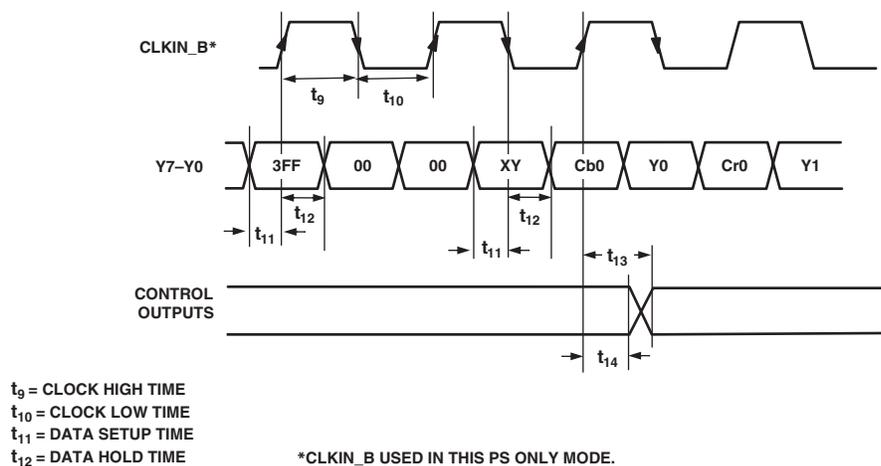
Figure 6. PS Only 4:2:2 1 × 8-Bit Interleaved at 27 MHz EAV/SAV Input Mode [Input Mode 100]
