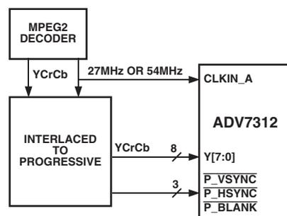
Figure 27. 1 × 8-Bit PS at 27 MHz or 54 MHz
