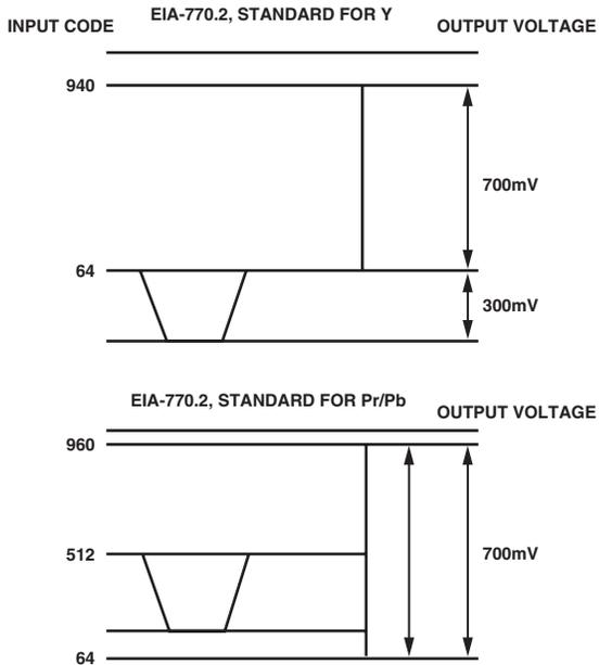
Figure 91. EIA 770.2 Standard Output Signals (525p/625p)
