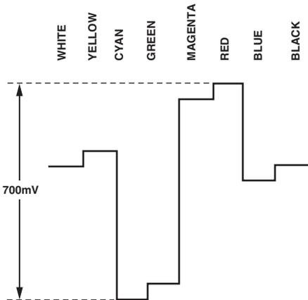
Figure 101. Pr Levels—NTSC
