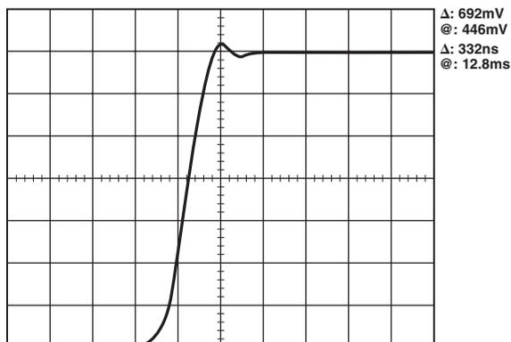
Figure 44. Input Signal to Adaptive Filter Control
