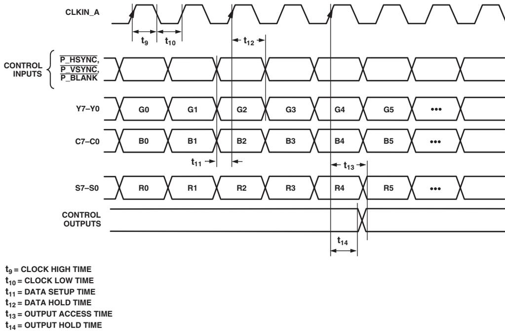
Figure 3. HD RGB 4:4:4 Input Mode [Input Mode 010]
