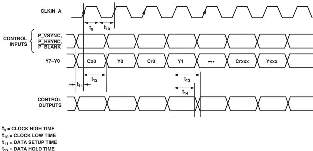
Figure 5. PS 4:2:2 1 × 8-Bit Interleaved at 54 MHz  $\overline{HSYNC}/\overline{VSYNC}$  Input Mode [Input Mode 111]
