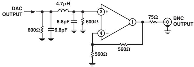
Figure 56. Example of Output Filter for PS, 8× Oversampling
