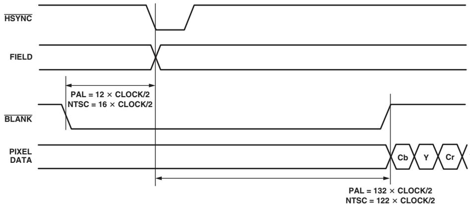
Figure 83. SD Timing Mode 1—Odd/Even Field Transitions Master/Slave
