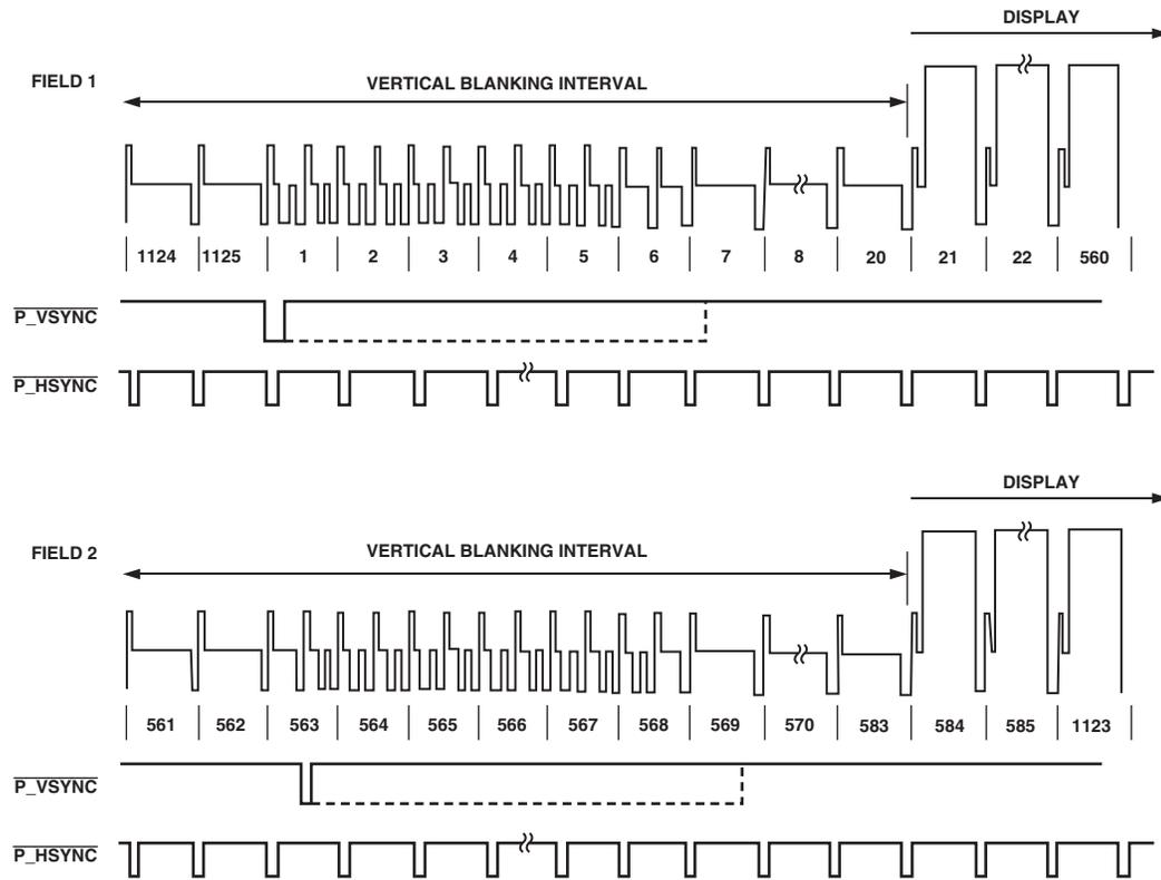
Figure 90. 1080i  $\overline{HSYNC}$  and  $\overline{VSYNC}$  Input Timing
