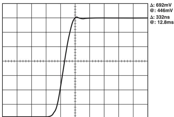
Figure 45. Output Signal after Adaptive Filter Control
