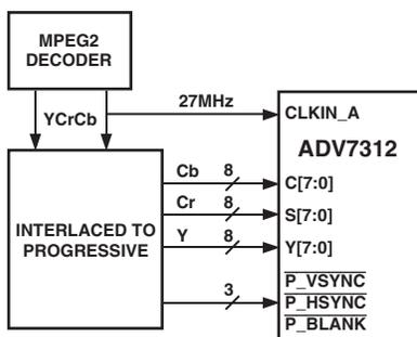
Figure 22. Progressive Scan Input Mode
