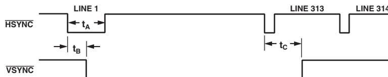
Figure 20. Timing Register 1 in PAL Mode
