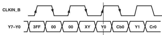
CLOCK EDGE ADDRESS 0x00 BIT 1 SHOULD BE SET TO 1 IN THIS CASE.
