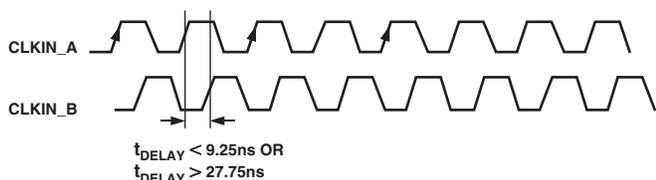
Figure 25. Clock Phase with Two Input Clocks
