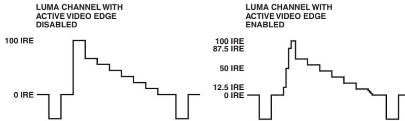
Figure 51. Example of Active Video Edge Functionality
