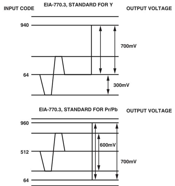
Figure 93. EIA 770.3 Standard Output Signals (1080i, 720p)
