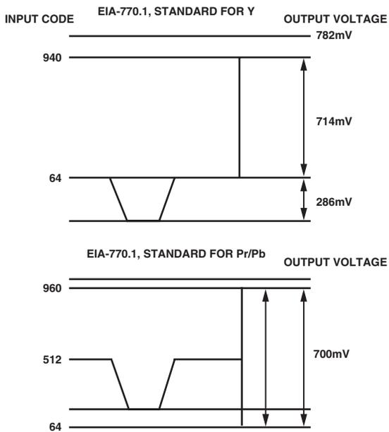
Figure 92. EIA 770.1 Standard Output Signals (525p/625p)
