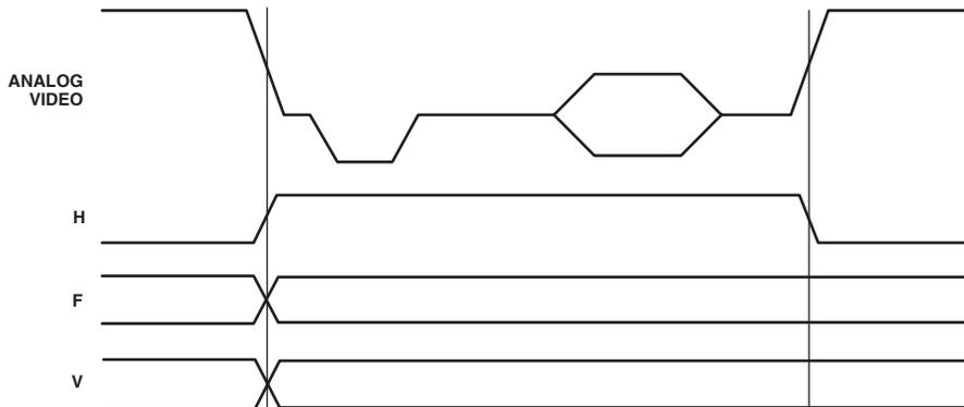
Figure 80. SD Master Mode 0, Data Transitions
