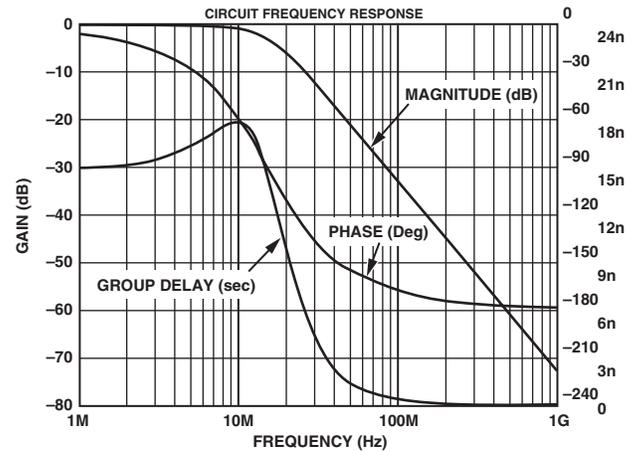
Figure 55. Filter Plot for Output Filter for SD, 16x Oversampling
