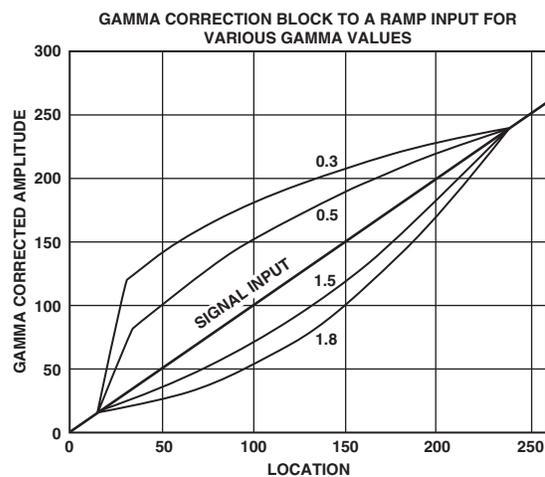
Figure 41. Signal Input (Ramp) and Selectable Output Curves
