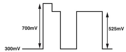
Figure 97. SD RGB Output Levels—RGB Sync Disabled
