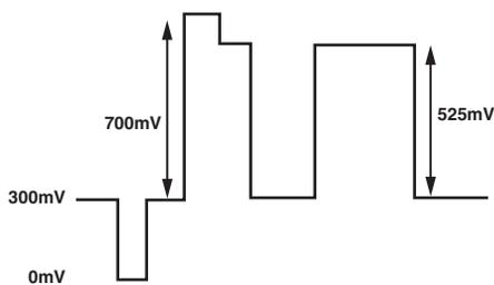
Figure 96. PS RGB Output Levels—RGB Sync Enabled
