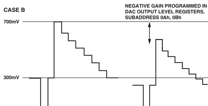
Figure 39. Programmable DAC Gain—Positive and Negative Gain
