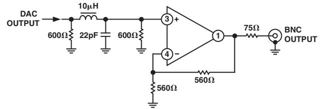
Figure 54. Example of Output Filter for SD, 16x Oversampling
