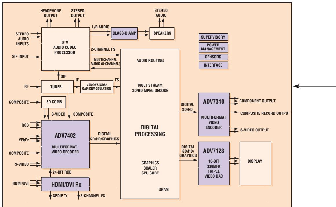
The ADV7402 and ADV7400 multiformat video decoders simplify front end digitizer and decoder architectures by reducing board space, simplifying auto detection and switching of inputs, and reducing overall system power consumption.
