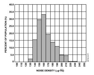
Figure 13. Y Axis Noise Density at 25°C
