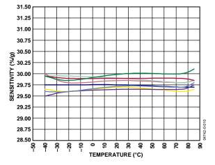
Figure 12. Sensitivity vs. Temperature – Parts Soldered to PCB
