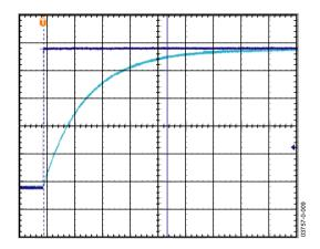
Figure 20. Turn-On Time –  $C_{X_r}C_Y = 0.1 \mu F$ , Time Scale = 2 ms/div
