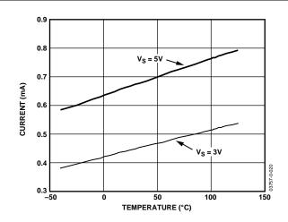
Figure 15. Supply Current vs. Temperature
