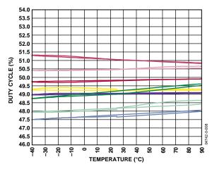
Figure 9. Zero g Bias vs. Temperature - Parts Soldered to PCB
