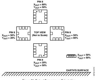
Figure 21. Output Response vs. Orientation
