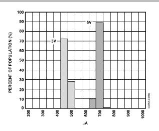
Figure 18. Supply Current at 25°C
