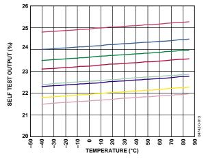
Figure 17. Self Test Response vs. Temperature
