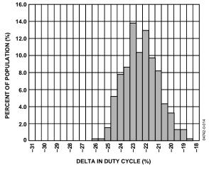
Figure 19. Y Axis Self Test Response at 25°C
