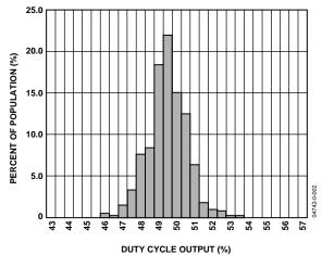
Figure 3. X Axis Zero g Bias Deviation from Ideal at 25°C
