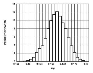
Figure 4. X-Axis Output Sensitivity Distribution at  $X_{OUT}$
