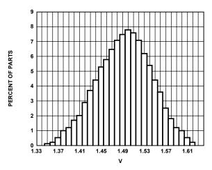
Figure 3. Y-Axis Zero g BIAS Output Distribution
