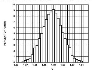
Figure 2. X-Axis Zero g BIAS Output Distribution
