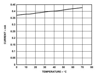
Figure 8. Typical Supply Current vs. Temperature
