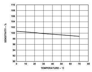
Figure 6. Normalized Sensitivity vs. Temperature
