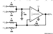
Where:  $V_0 = V_1 + V_2 - V_3 - V_4$  $(V_1 + V_2 \ge (V_3 + V_4) \text{ to keep } V_0 > 0V_{DC}$
