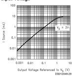
Sinking Current vs Output Voltage
