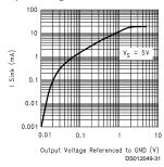
Sinking Current vs Output Voltage
