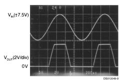
FIGURE 2. A ±7.5V Input Signal Greatly Exceeds the 5V Supply in Figure 3 Causing No Phase Inversion Due to R
