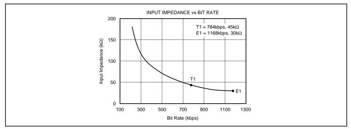
CURVE 3. Input Impedance of rxLINE and rxHYB.
