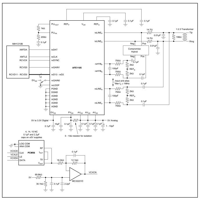
FIGURE 2. Basic Connection Diagram.
