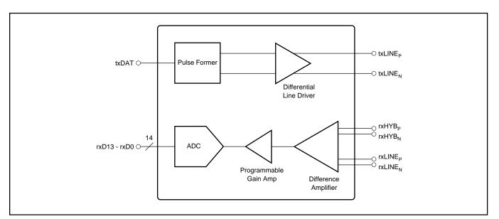
FIGURE 1. Functional Block Diagram of AFE1105.
