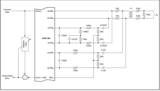
FIGURE 4. Uncancelled Echo Test Diagram.
