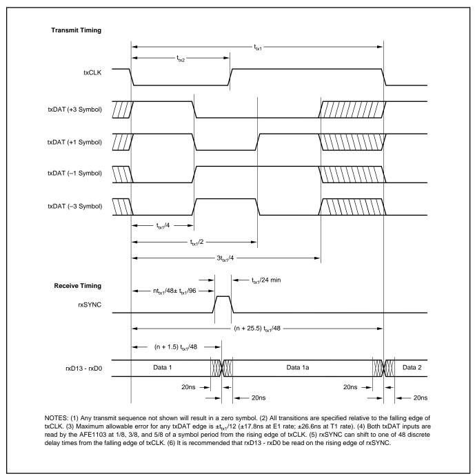
FIGURE 3. Timing Diagram.
