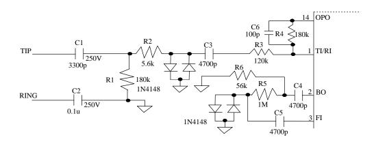
In the application circuit above, some of the external element values are crucial. C2 value could not be less than 0.1uF. R2 = 5.6k is proper and you had better not to change it. The diode has to use Si type diode for noise consideration.
