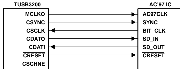
Figure 2–2. Connection of the TUSB3200A to an AC '97 Codec
