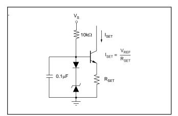
FIGURE 2. REF1112 Provides a Stable Current Source.
