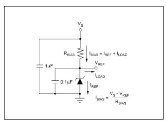
FIGURE 1. Typical Connections.
