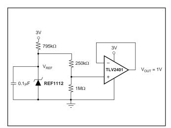
FIGURE 3. MicroPOWER 3µA 1V Voltage Reference.
