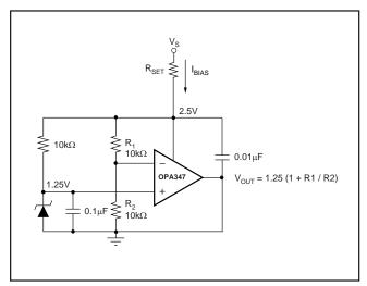
FIGURE 5. Adjustable Voltage Shunt Reference
