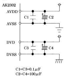
To use the same supply for both digital and analog power supply (DVDD and AVDD), insert  $10\,\Omega$  resistor between AVDD and DVDD. AVSS and DVSS must be separated on the board, and connected them at power supply unit.
