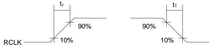
Fig. 12 Signal Rise and Fall Characteristics
