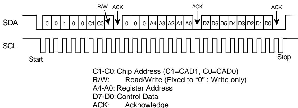
\* When the AK4363 is in the power down mode (PDN = "L") or the MCLK is not provided, writing into the control register is inhibited.
