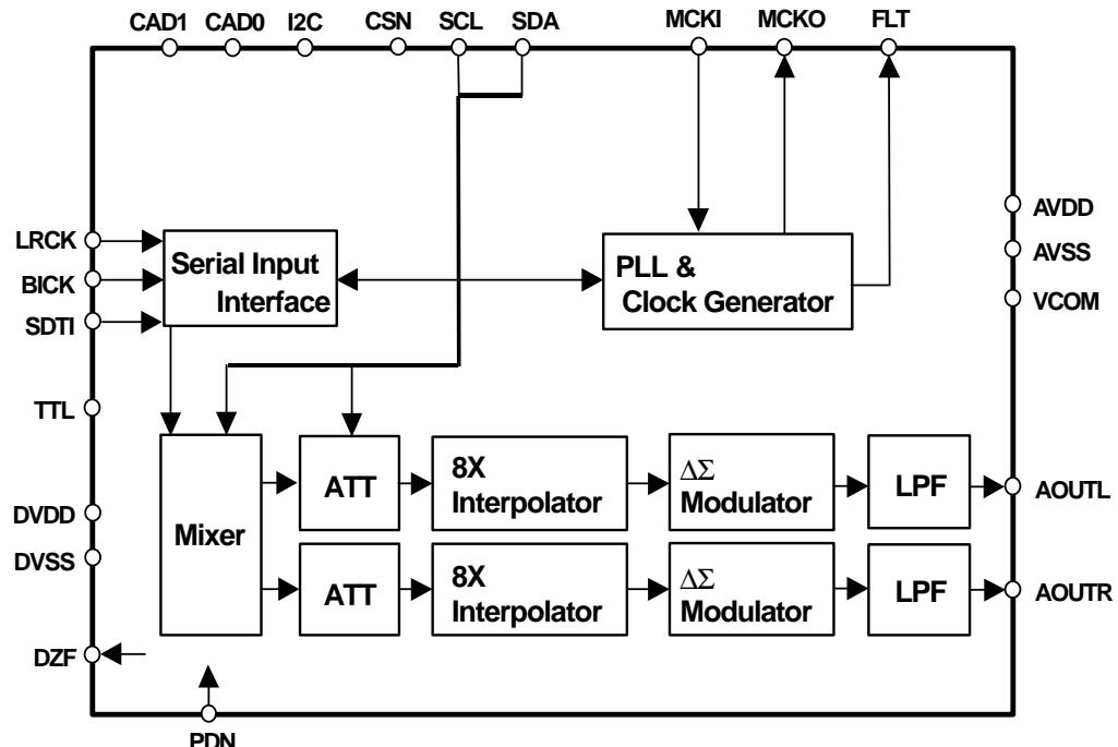
Figure 2. I<sup>2</sup>C Bus Control Mode (I2C = "H")
