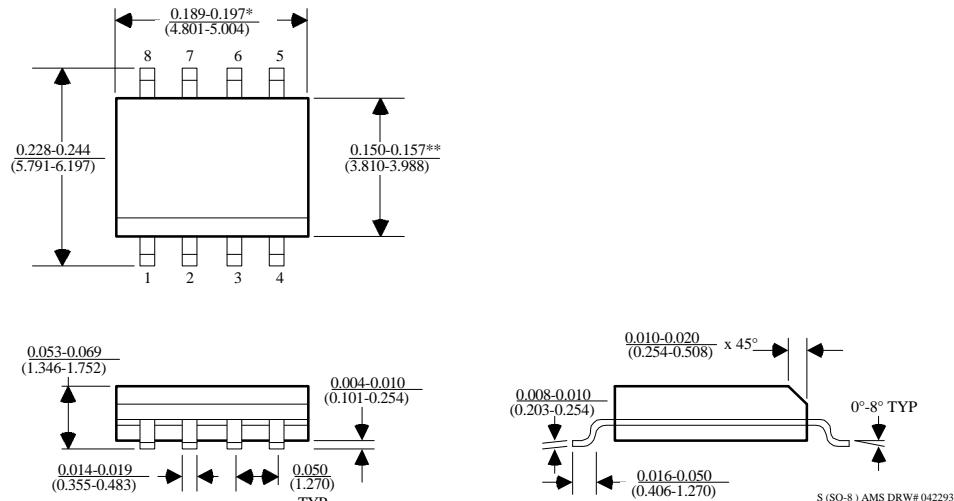
\*DIMENSION DOES NOT INCLUDE MOLD FLASH. MOLD FLASH
