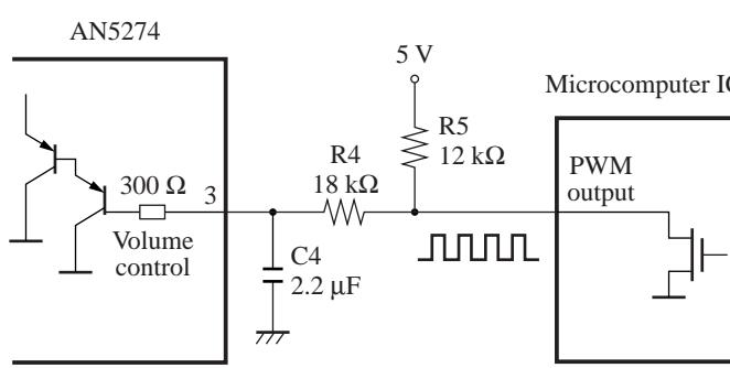
Fig. Volume control interface circuit for AN5274
