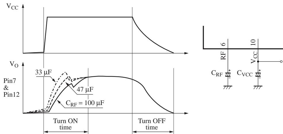
The turn ON time in the AN5274 is determined by the capacitance value of  $C_{RF}$ . If value of the  $C_{RF}$  is smaller,  $V_O$  will turn on faster.
