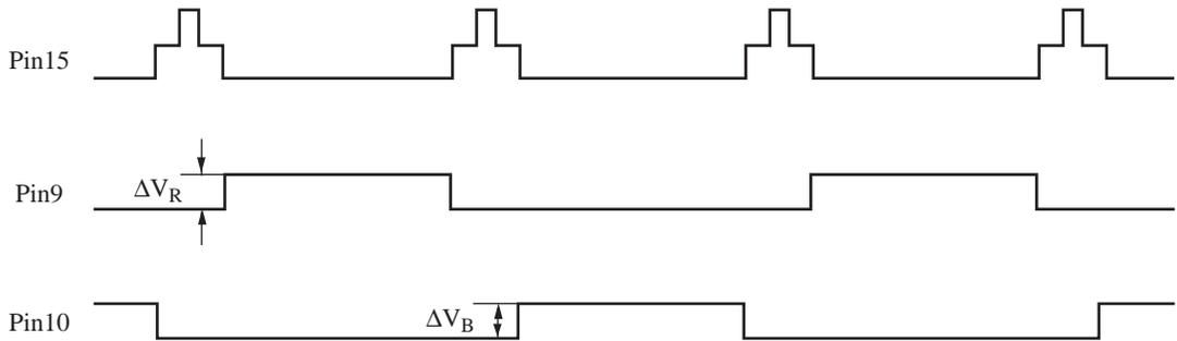
Input 100 % white signal and adjust the voltage of Pin4 so that  $\Delta V_B$  becomes 0 mV. Let the adjusted voltage be  $V_{AD4}$ .
