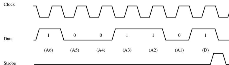
1. Data is read into the shift register in synchronization with a rising edge of the clock, with the higher data being shifted sequentially on a first-come highest-bit basis.
