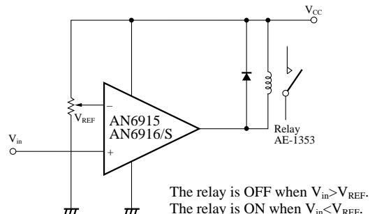
The relay is OFF when  $V_{in} > V_{REF}$ .
