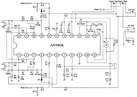
Note: Resistors R11/R12 and diodes D1/D2 are used to mute pre-amp during radio mode. Resistor R13/R14 act as multiplexer load.
