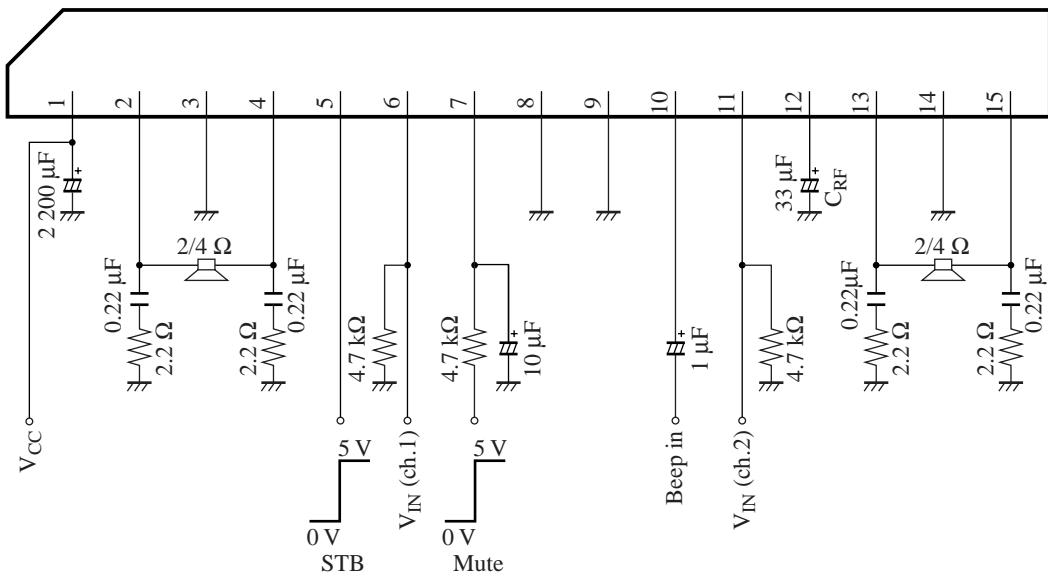
Note) Standby state when STB pin is open-circuit.
