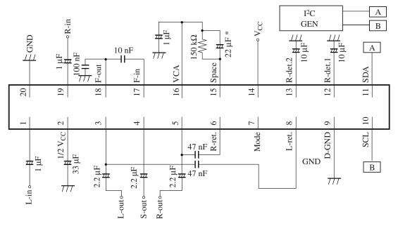
Note) When switching noise occurs at mode switching, insert a capacitor between pin 7 and GND.
