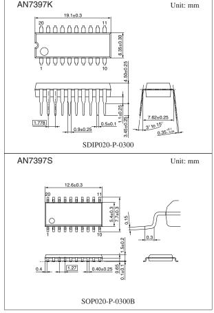
Note) The packages (SDIP020-P-0300 and SOP020-P-0300B) of this product will be changed to lead-free type (SDIP020-P-0300A and SOP020-P-0300E). See the new package dimensions section later of this datasheet.
