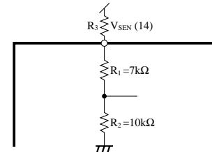
However, take care that an external resistance causes different temperature characteristics.
