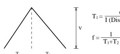
$T_1 = \frac{CV}{I \text{ (Discharged)}} \quad T_2 = \frac{CV}{I \text{ (Charged)}}$ $f = \frac{1}{T_1 + T_2}$ <div style="border: 1px solid black; padding: 5px; margin-left: 20px;">       I Discharged=52μA<br/>       I Charged=30μA<br/>       V=0.58V     </div> <p style="text-align: right;">In normal mode</p> |
