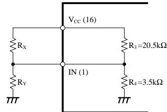
2. Method for making decreased voltage detection variable
