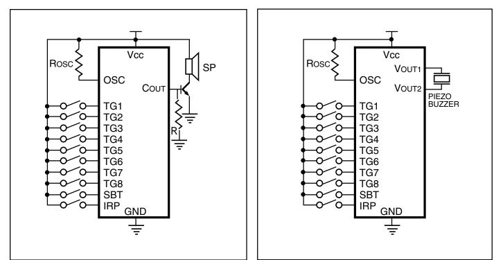
Figure 1. Typical Application with Speaker
